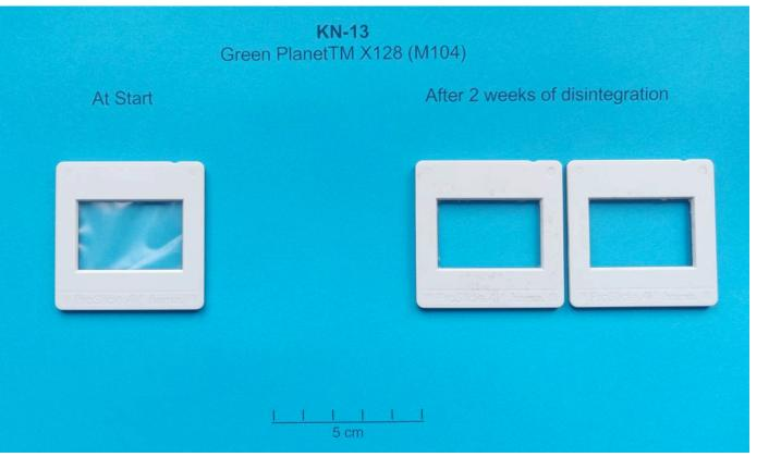
Qualitative disintegration test under high solid anaerobic digestions / modified ISO 15985) Mesophilic (37 +/- 2°C) Visual monitoring after 14 days;28 days,... (Test Facility by OWS)
